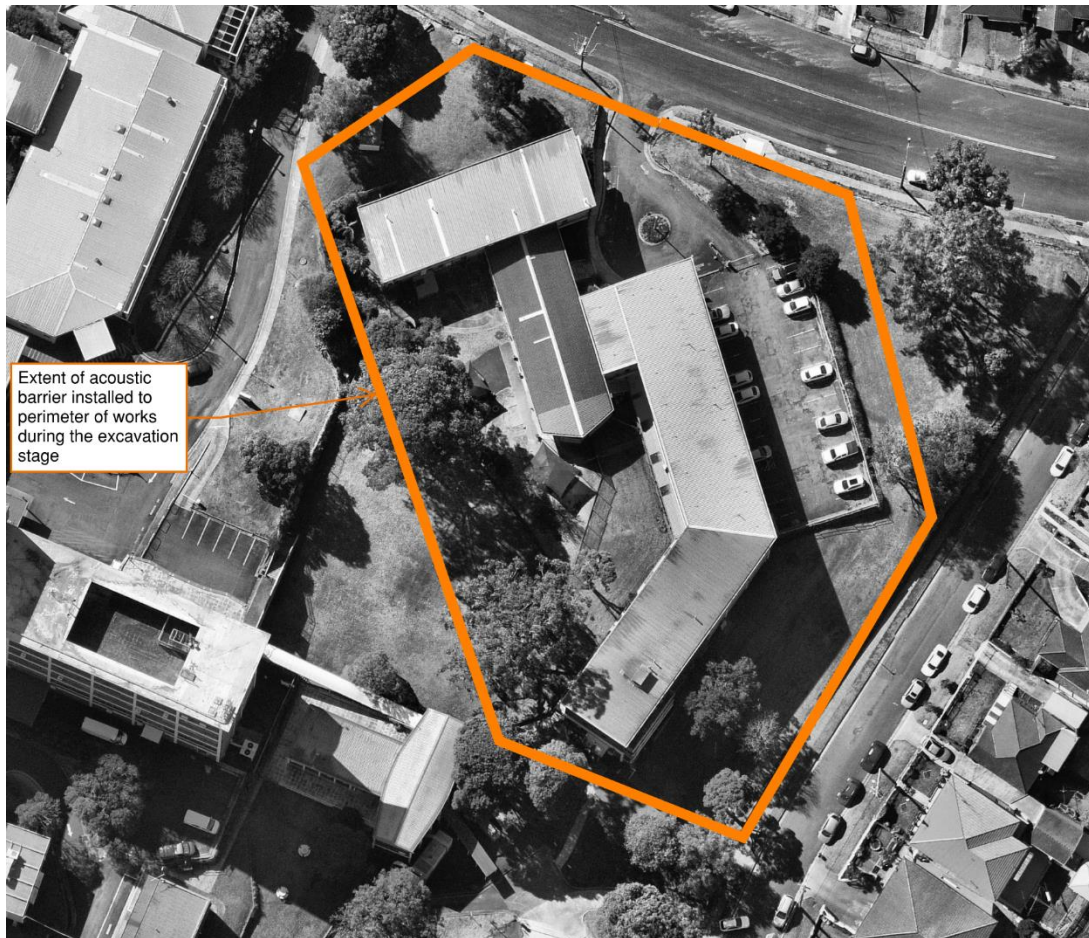
Figure 4: Extent of acoustic barrier (A-Class or B-Class Hoarding)
